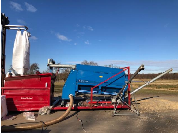
Photo 1. Kongskilde rotating cleaner with 3 different sieves and air suction. The unit is fitted with a hopper on the lefthand side and two augers – one for each separated part. Photo: Visti Møller, Buurholt.
