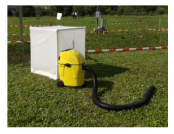
**Biocoenometer (suction sampler).** Allows volume-specific sampling but is rather labour-intensive. [Images: CS]
