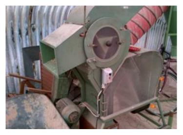
**Threshing machine** for small-scale threshing of manually harvested material. [Photo: CS]
