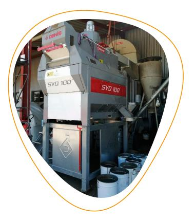
Fig. 4. Vibrating cleaner SVD100 from Etablissements Denis used to demonstrate the feasibility of the separation of species mixture and the resulting economic benefit (Picture from Patrick Bourachot)
