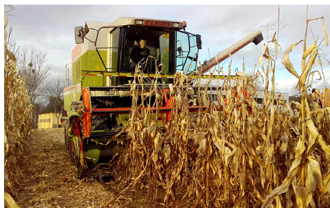
Fig. 2 Harvesting a bean-corn plant team with a combine harvester for wheat
