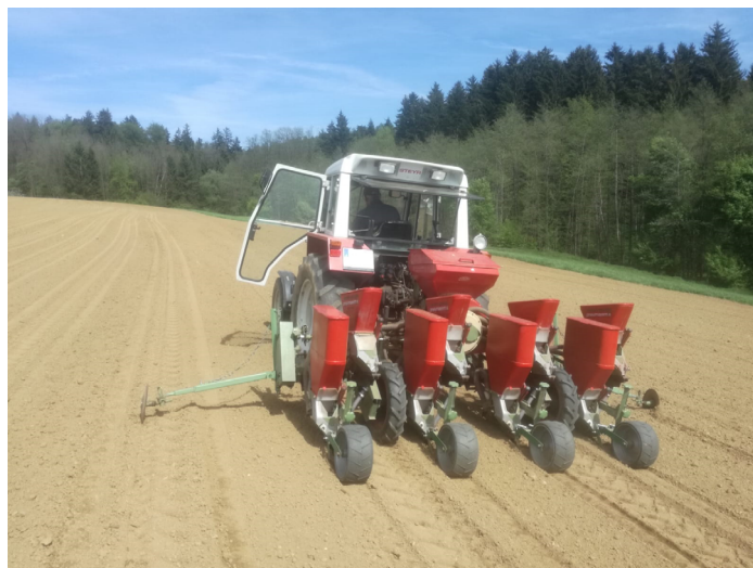
Fig. 1 Consider all options when using plant teams. For example, a drill with separate seed tanks can be used for plant team components with different seed sizes.
